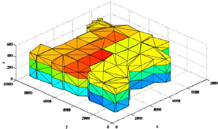
**Figure 2:** Unstructured (voronoi) grid shaded by cell index.
